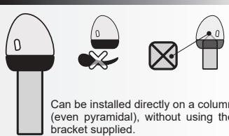
Can be installed directly on a column (even pyramidal), without using the bracket supplied.
