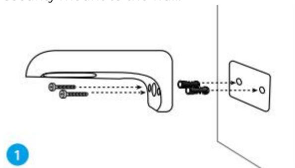
**Note:** Use the drywall anchors included in the package if needed.
