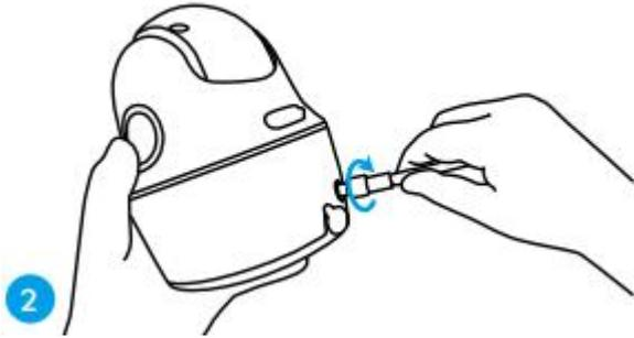
**Note:** In order to get a better network connection, it is recommended to install the antenna upward or horizontally.
