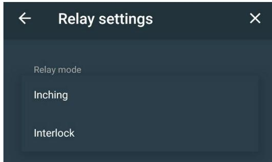
An **option to set the duration of inching interval** is available in inching mode.
