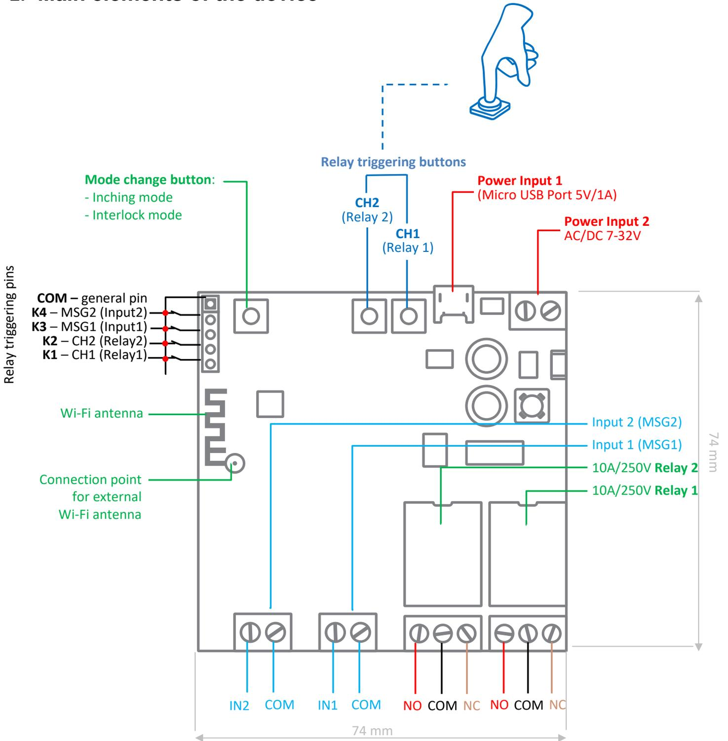
**Power connectors** - the relay is powered by connecting AC / DC 7-32V power supply or a power supply unit with a Micro USB connector.
