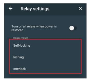
An **option to set the duration of inching interval** is available In inching mode.
