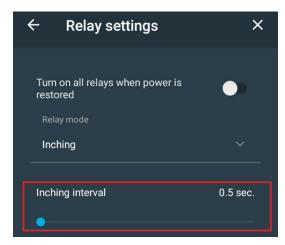
"Turn on all relays when power is restored" - activating this option allows you to keep the relay in its last state when the power is turned off and then turned on. By default, this option is inactive, therefore, when the power supply is turned off and then turned on, the relays will remain disabled.
