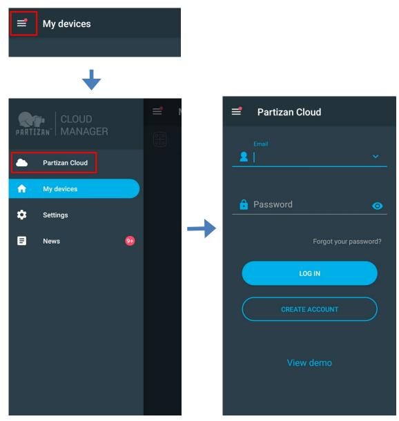
After signing into the cloud account you can go directly to device setting.
