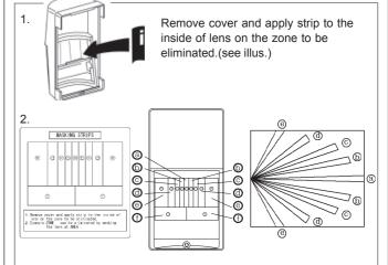
Example: ZONE "a" can be eliminated by masking the lens at area "a" (see illus.).
