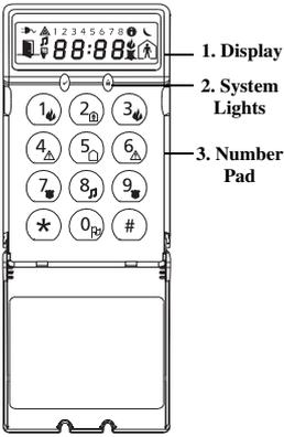
The LCD5511 shows the status of your security system using an LCD display, along with fixed symbols and numbers.
