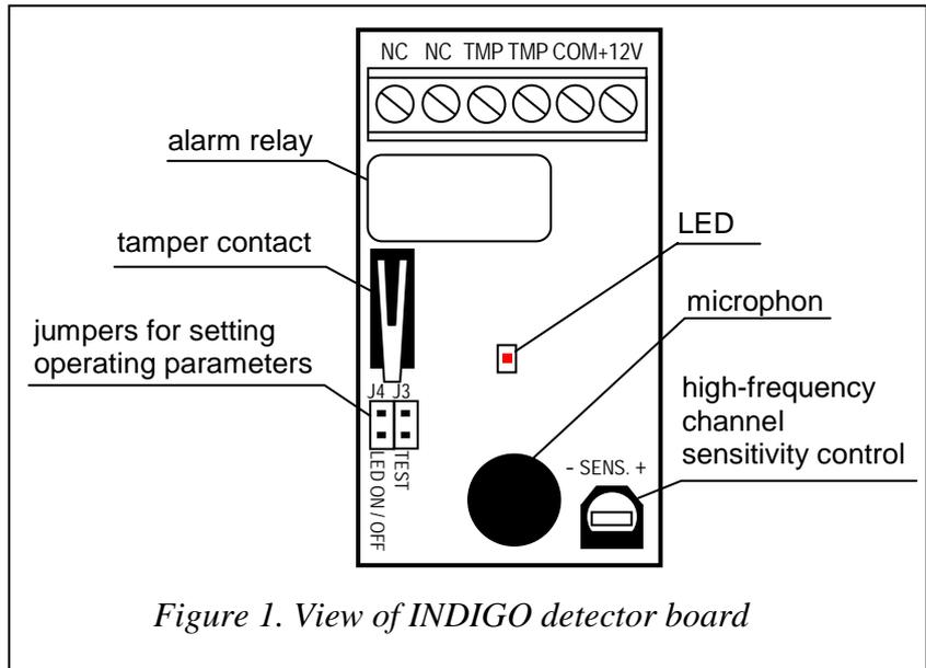
*Figure 1. View of INDIGO detector board*
