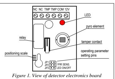
Three pairs of pins are used to set the detector working parameters (see Table)
