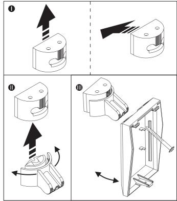
Figure 3. Mounting the detector on the holder.
