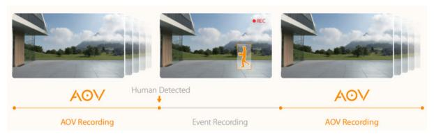
AOV PT takes it to the next level with the latest Always-on Video (AOV) technology. With AOV, the camera intelligently allocates its resources by compiling time-lapse videos from images captured at your scheduled intervals. Additionally, it also records full videos when an alarm is triggered, precisely controlling the power consumption for each operation. This enhances home safety while reducing battery consumption.
