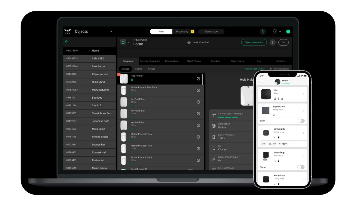
All types of Ajax apps connect to a hub using a secure channel with Ajax Cloud — our server solution located at several AWS data centres. All security system settings are always available in the app. Even when PRO is far away from the facility, he can connect CCTV cameras, add users, test radio signal level, create security groups and scenarios, or connect a hub to an alarm monitoring company.
